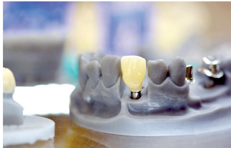
Additive manufacturing – or 3D printing – unlocks new possibilities for chairside manufacture of dental components.
